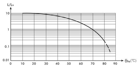
L<sub>N</sub>: Expected life at 70°C hot spot temperature L: Expected life at θ<sub>hs</sub> hot spot temperature
